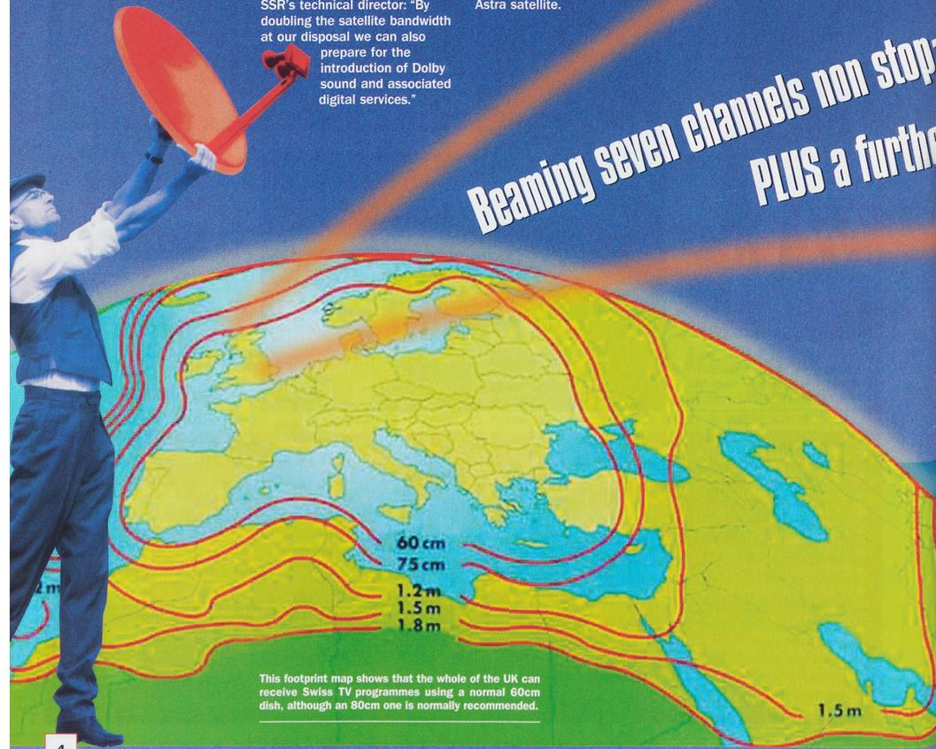
This footprint map shows that the whole of the UK can receive Swiss TV programmes using a normal 60cm dish, although an 80cm one is normally recommended.
