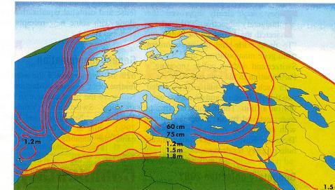
The reception range of SBC programmes and the satellite-dish diameter required.
