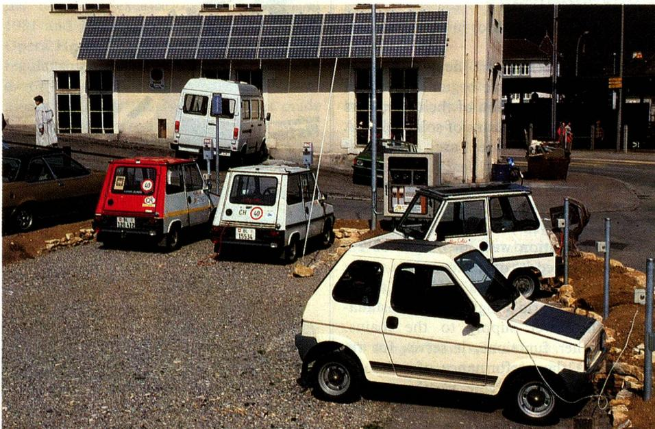
*How electrically powered motor cars can refuel. (Photo: Dominik Labhardt)*
