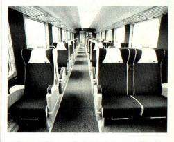
pull-out tables, upholstered seats and backrests. The assembly is screwed together by hand. The pivotal points for movement are indicated by clearly visible articulations. Even the upholstery material is specially woven with front and back in different colours, and mechanically interlocked. The principle is the same for both seats and wall: the construction and the mechanical fastening must be recognisable.
