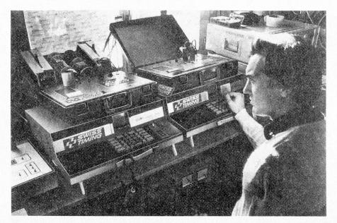
less than 1/1000 second over the space of 24 hours. Considering that most races only last for a few minutes, this gives an idea of the accuracy provided. Moreover, the capactiy of this equipment is far from being wholly used. In fact, all the times are registered to a thousandth of a second but only given to a hundredth, in accordance with the rules of the various sports federations.
