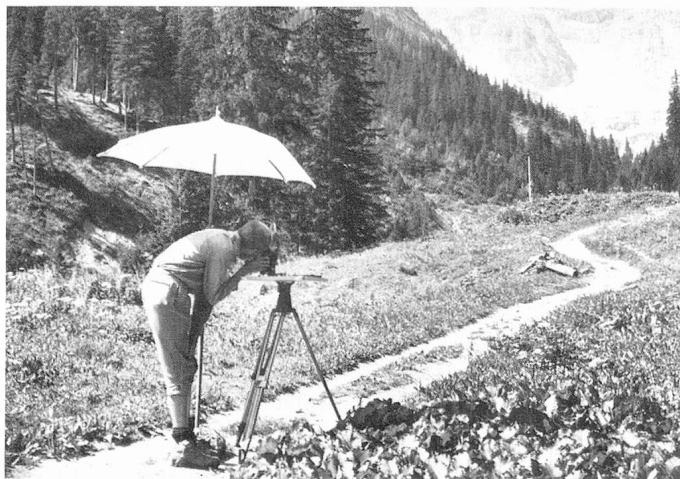
Topographical details were surveyed using the planetable
