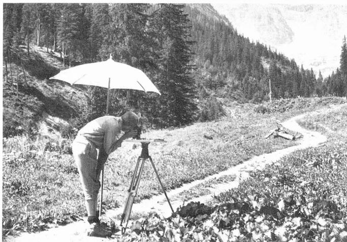
Topographical details were surveyed using the planetable
