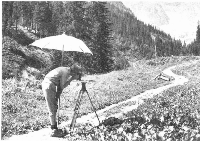
Topographical details were surveyed using the planetable
