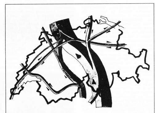
The St. Gothard Pass, linking the northern and southern parts of the European Community. Today, there is no need to prove the importance of this route which was opened in about 1240. The thickness of the lines shows the relative density of rail traffic. On the St. Gothard line 200 to 300 trains pass daily. Since saturation point has been reached a new tunnel is being built.
