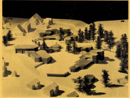
School project at Zurich-Witikon. Arch.: Roland Gross. Hierarchic plan: two classrooms form a group and two and three groups constitute a school building. The rooms shared by the two schools - examples 4 and 5 - are centrally situated.
