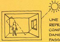
UNE FENETRE CONVENABLEMENT ORIENTEE REPRESENTE UN CAPTEUR SOLAIRE. COMPLETEE D'UNE MASSE THERMIQUE INTEGREE DANS LA STRUCTURE, ON OBTIENT UN SYSTEME PASSIF DU TYPE SOLEIL → ESPACE. LES MURS ET LES PLANCHERS REMPLISSENT UNE DOUBLE FONCTION : ILS DEVIENT ELEMENTS PORTEURS + ACCUMULATEURS THERMIQUES.
