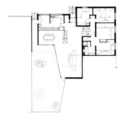
Type FC/5 Residential surface 90.41 m² Constructed volume 407.62 m³ Net building site 183.71 m²
