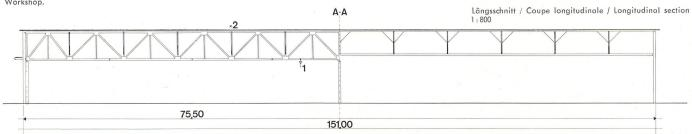
1 Genieteter Stoß / Joint riveté / Riveted joint 2 Geschraubter Stoß / Joint vissé / Screwed joint
