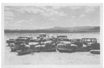
Figure 5.96a. Effect of nuclear explosion on automobiles in simulated parking lot, Nevada Test Site. Much of the damage to glass, paint, and interiors was due to fires caused by thermal radiation.
