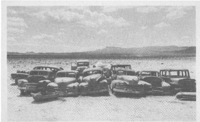
Figure 5.96a. Effect of nuclear explosion on automobiles in simulated parking lot, Nevada Test Site. Much of the damage to glass, paint, and interiors was due to fires caused by thermal radiation.
