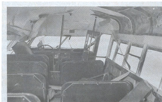
Figure 5.96d. Interior damage to bus shown above, caused by blast, displacement, and fire.
