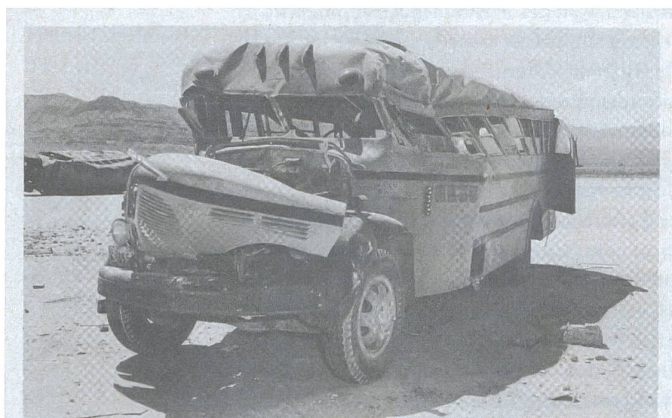
Figure 5.96c. Typical public bus damaged by a nuclear explosion, Nevada Test Site; this bus, like the one in the left background, was overturned, coming to rest as shown after a displacement of 50 feet.
