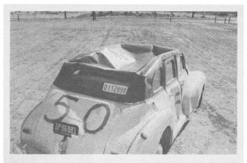
Figure 5.96b. Damage to automobile originally located behind wood-frame house (5 psi overpressure); the front of this car can be seen in Figure 5.14. Although badly damaged, the car could still be driven after the explosion.
