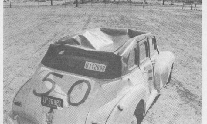
Figure 5.96b. Damage to automobile originally located behind wood-frame house (5 psi overpressure); the front of this car can be seen in Figure 5.14. Although badly damaged, the car could still be driven after the explosion.
