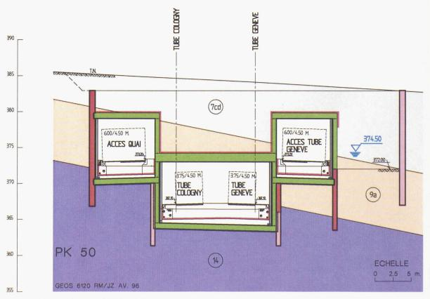
Figure 3. - Ouvrage de raccordement: coupe
