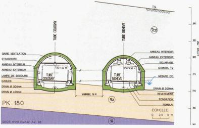
Figure 5. - Tunnel: profil normal
