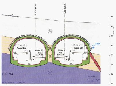
Figure 4. - Tunnel: profil de transition
