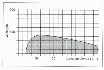
Fig. 5. - Spectre de la radiation terrestre, ciel clair [1].
