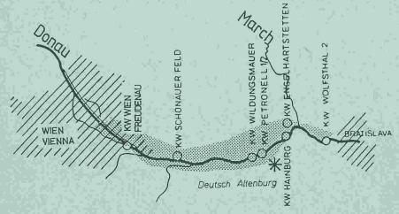
Fig. 2 Alternative plans for hydropower utilization
