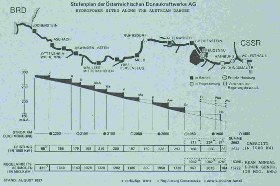
Fig. I Hydropower utilization along the Danube in Austria
