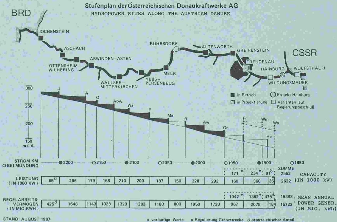
Fig. 1 Hydropower utilization along the Danube in Austria
