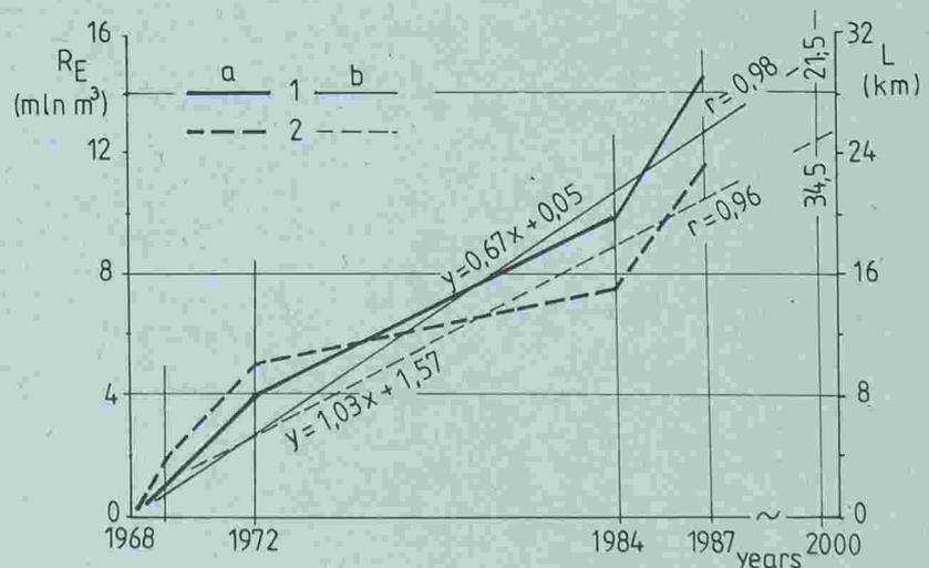
Fig. 1. The balance of the bed erosion  $-R_E$  (1a) and the rate of the front of erosional zone shifting  $-L$  (2a) downstream from the Wloclawek dam between 1968-1987, and its straight regression until 2000 (1b and 2b respectively).
