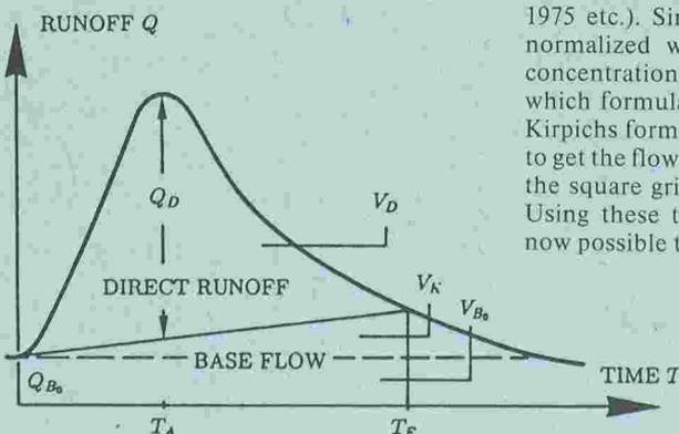
Fig. 2 Characteristic parameters of a flood event
