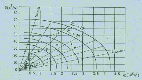
Fig. 1 "Design curves": Lines of constant bivariate probability of  $V_D$ ,  $Q_D$  (probability of occurance of  $V_D$ ,  $Q_D$  in the upper right quadrant).
