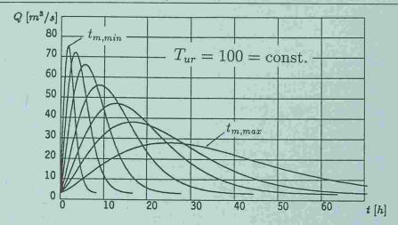
Fig. 2 "Design hydrographs": Flood hydrographs of constant bivariate probability.
