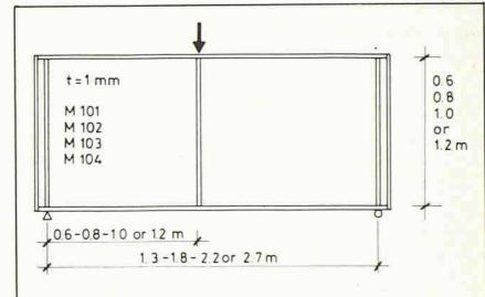
Fig. 3. — Main dimensions of test girders, series M.
