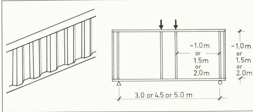
Fig. 1. — Main dimensions of test girders, series L.
