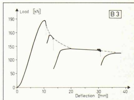
Fig. 5. — Load versus deformation diagram of girder B3.
