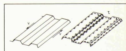
Fig. 4. — Part of trapezoidal panel under shear.
