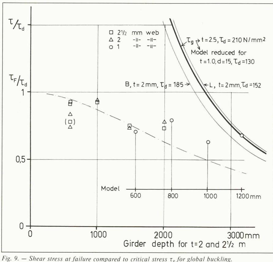
Fig. 9. — Shear stress at failure compared to critical stress  $\tau_g$  for global buckling.
