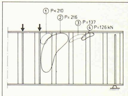
Fig. 6. — Buckling propagation of girder B4b.
