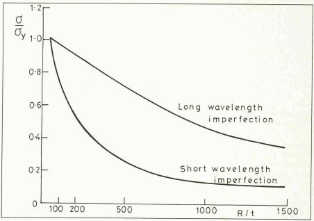
Figure 3. — Effect of longitudinal imperfection wavelength on strength.
