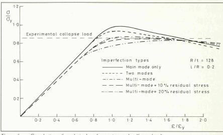
Figure 6. - Correlation of analytical and experimental collapse loads.
