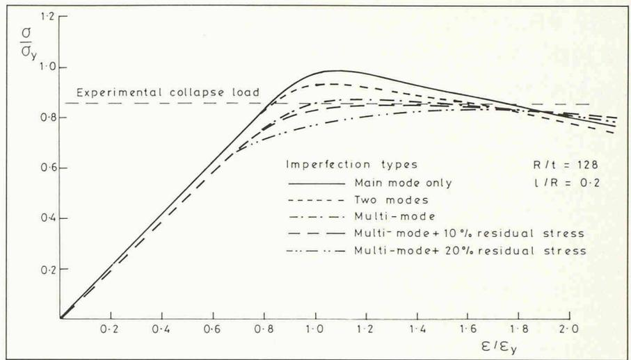
Figure 6. — Correlation of analytical and experimental collapse loads.
