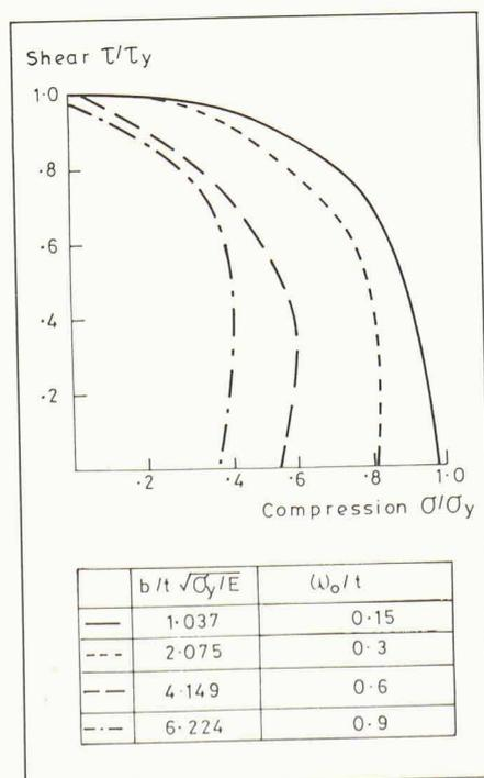
Figure 1. — Interaction of compression and shear on square plate panels.
