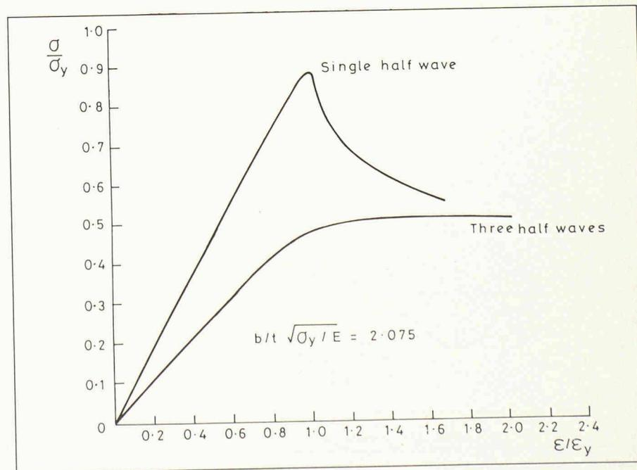
Figure 2. — Effect of imperfection form on compressive strength.
