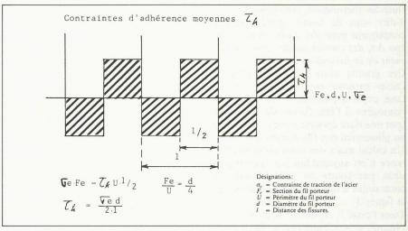
Fig. 3. — Fissuration.
