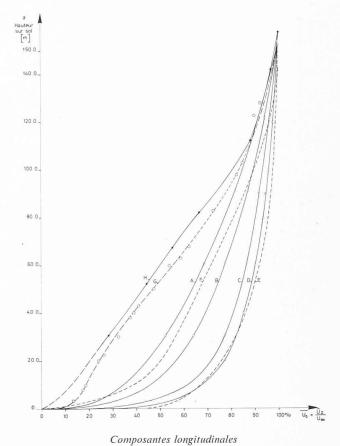
ABC  $\frac{\overline{u}_z}{\overline{u}_\infty} = \left(\frac{Z}{Z_0}\right)^{\alpha}$   $Z_0 = 152,4 \text{ m}$
