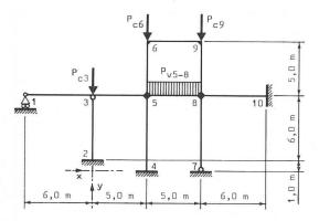
$$\begin{array}{c} J_{1\text{-}3} = J_{3\text{-}5} = J_{6\text{-}9} = J_{8\text{-}10} = 5000 \text{ cm}^4. \\ J_{2\text{-}3} = J_{5\text{-}6} = J_{5\text{-}8} = J_{8\text{-}9} = 15\ 000 \text{ cm}^4. \\ J_{4\text{-}5} = J_{7\text{-}8} = 20\ 000 \text{ cm}^4. \end{array}$$
