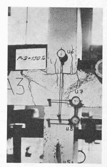
Fig. 10. — Eprouvette A 3; charge verticale: 380 t.
