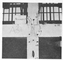
Fig. 11. — Eprouvette A 3; charge verticale: 483 t, charge de rupture.
