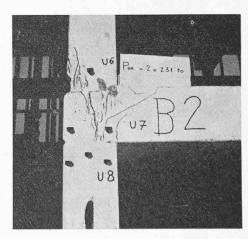
Fig. 19. — Eprouvette B 2; charge verticale: 462 t, charge de rupture.
