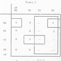
$Z = a + b c d + \overline{b} \overline{c} \overline{d}$
