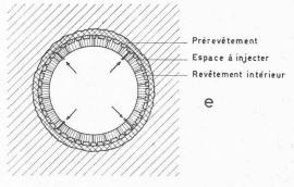
EXPANSION CHEMISES EN TÔLE AU-DELÀ DE LA LIMITE D'ÉLASTICITÉ
