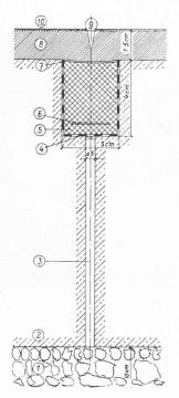
Fig. 13. — Joint de dilatation. Echelle 1: 2.
