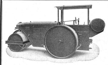
Rouleau Ammann - trijante Diesel, charge utile 3 - 14 tonnes
