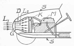
$\begin{array}{ll} {\rm Fig.~5. \ --- \ R\'efrig\'eration~syst\`eme~Jaray.} \\ L_1 = {\rm courant~d'air. \ ---} G = {\rm grille~de~protection. \ --} D = {\rm buse.} \\ --- L_2 = {\rm trajectoires~des~filets~d'air~dans~la~buse. \ ---} K = {\rm radiateur. \ ---} M = {\rm moteur. \ ---} S = {\rm carrosserie.} \end{array}$
