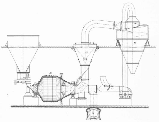
$\label{eq:figeneral} \begin{aligned} & \text{Fig. 2.} & -- \text{Installation de mouture crue.} \\ \textit{L\'egende.} & -- a = \text{moulin}; \ b = \text{foyer}; \ c = \text{soufflerie}; \ d = s\'e\text{parateur}; \ e = \text{cyclone.} \end{aligned}$
