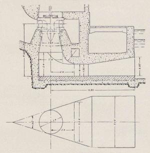
Fig. 7. — Coude Kaplan sur turbine  $K^n$  stinehamn. H = 10,55 m; P = 4100 ch; n = 214 t:  $\min$ ;  $n_s = 722$ .
