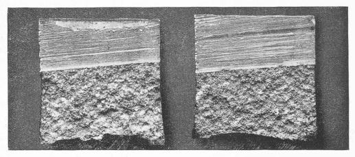
$\begin{array}{cccc} \text{Alliage: Aluminium} & 88 \% \\ * & \text{Zinc} & 10 \% \\ \text{Cuivre} & 2 \% \end{array}$
