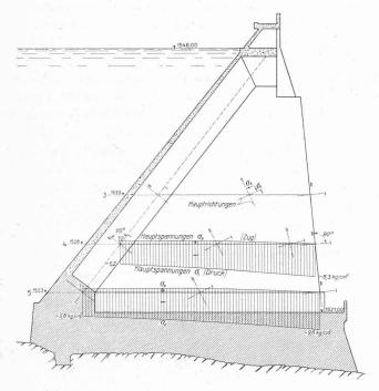
Fig. 15. — Diagramme des fatigues principales.  $\sigma_I = \text{Compression.} - \sigma_{II} = \text{Traction.} - I \text{ et } II = \text{Directions principales.}$
