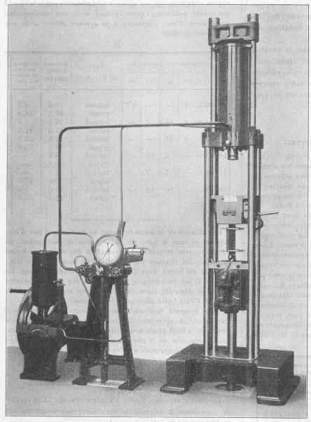
Fig. 4. Machine de traction, 50 T.
