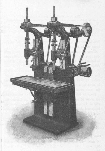
Fig. 7. — Perceuse sensitive rapide.
