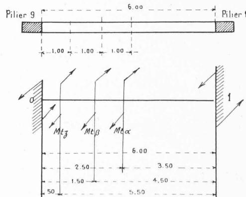
$$Mt_a = Mt_\beta = 1.45 \times 1.69 \text{ t.} + \frac{1.02 \text{ t.} \times \frac{1.45}{2}}{2} = 3.63 \text{ mt.}$$
