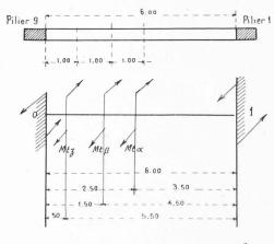
$$Mta = Mt\beta = 1.45 \times 1.69 \text{ t.} + \frac{1.02 \text{ t.} \times \overline{1.45}^2}{2} = 3.63 \text{ mt.}$$
