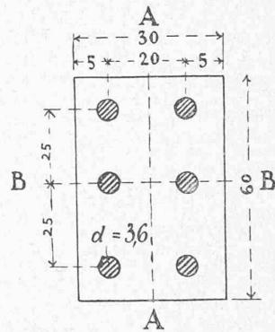
$$\begin{aligned} \text{Section } F &= 30 \cdot 60 + 10 \cdot 6 \cdot \pi \cdot 4,8^2 \\ &= 1800 + 611 = 2411 \text{ cm}^2. \end{aligned}$$
