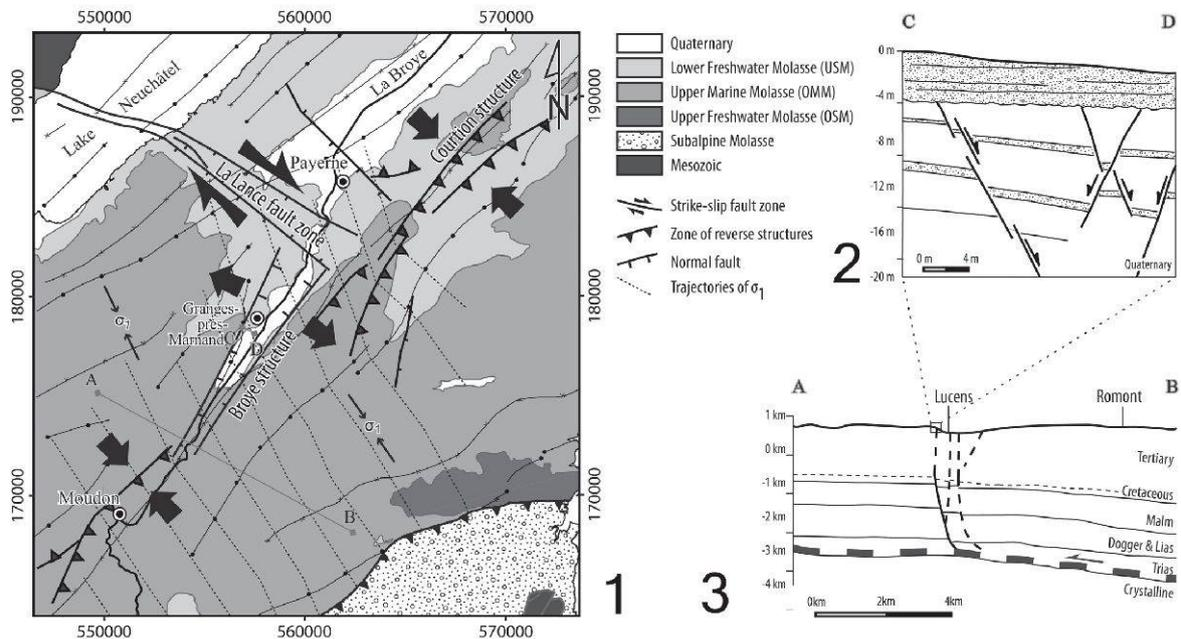
Figure 1.–Interpretation model of the Broye Graben System.
