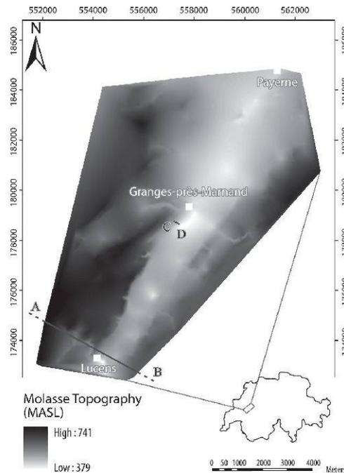
Figure 5.–Molasse topography of the Broye valley with profiles A-B and C-D (figure 1). The colour grading from black (high) to white (low) indicates the altitude of the top of the Molasse in meters above sea level. The break in molasse topography of the northwestern slope of Broye valley is particularly well marked. The map was generated with the Esri ArcGIS Software by contouring of subsurface information from borehole data. The kriging method was used for interpolation.
