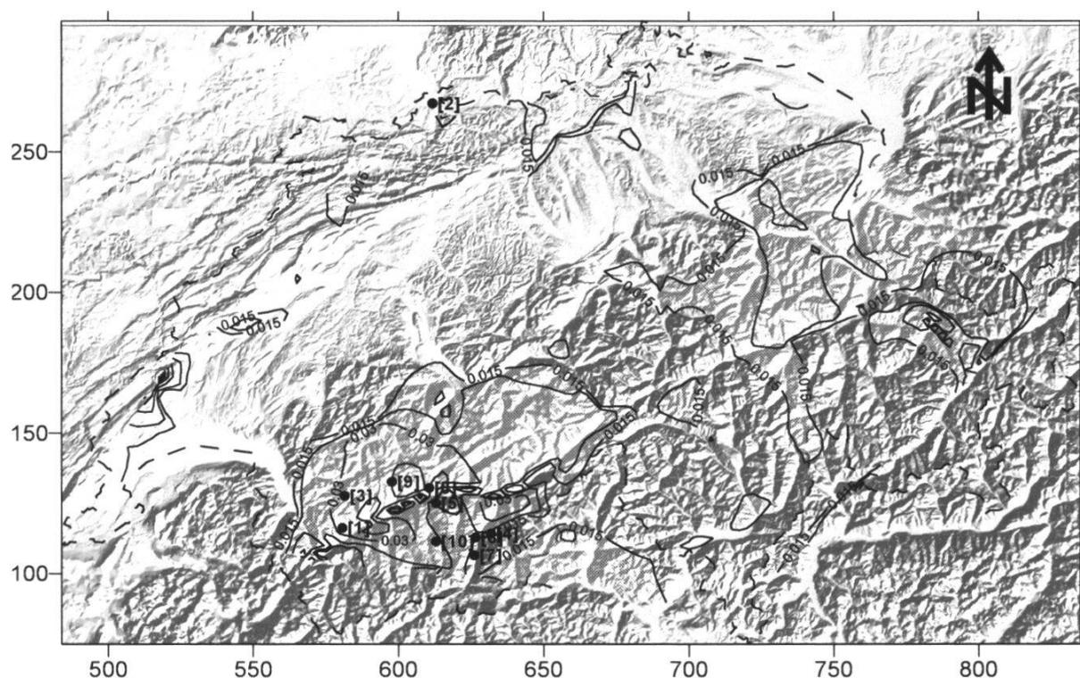
Figure 7.—Contouring of the gradient vector norm above  $0.015 \text{ mm km}^{-1} \text{ years}^{-1}$  and rockslide location in Valais (black points). The numbers in bracket indicate the related lines in Table 1. The point in Basel is not a particular location of one rockfall but indicate that many rockfalls are reported for the 1356 earthquake. (DEM RIMINI Federal Office of Topography (DS 033032)).
