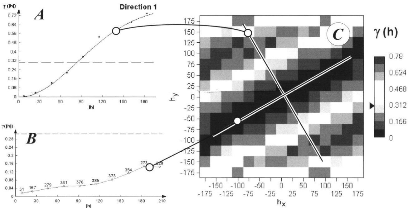
Figure 2.—(A) Variogramm for  $150^\circ$  direction displaying the greatest variability and model using two Gaussian components. (B) Variogramm perpendicular to A indicating the smallest variability. (C) Variographic surface of the uplift showing the great variability across the chain.
