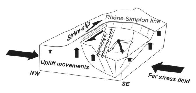
Figure 10.–(A) Schematic illustration of the Rhône-Simplon line system and the uplift movements.
