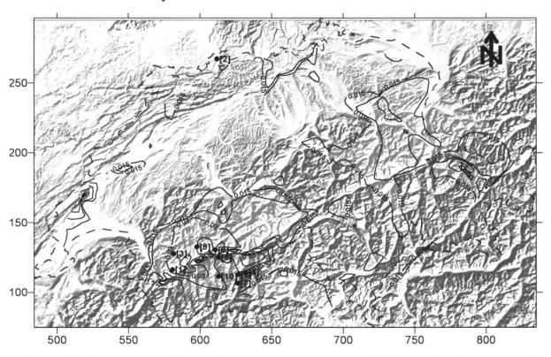
Figure 7.—Contouring of the gradient vector norm above 0.015 mm km<sup>-1</sup> years<sup>-1</sup> and rockslide location in Valais (black points). The numbers in bracket indicate the related lines in Table 1. The point in Basel is not a particular location of one rockfall but indicate that many rockfalls are reported for the 1356 earthquake. (DEM RIMINI Federal Office of Topography (DS 033032)).
