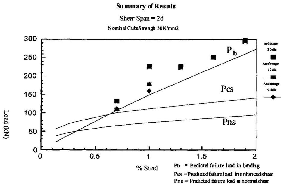
Figure 1 Comparison of Actual to Predicted Failure Loads
