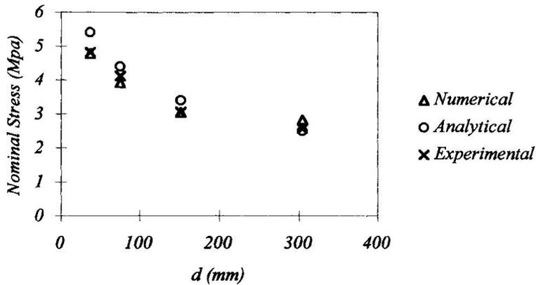
Fig. 1 Results on size effect for three-point bend notched beam
