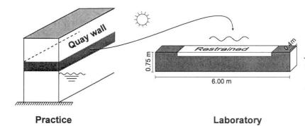
"Presentation of practice oriented full scale experimental research and the restrained temperature induced deformations at the top of the beam"
