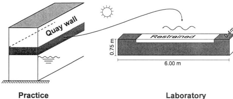
*"Presentation of practice oriented full scale experimental research and the restrained temperature induced deformations at the top of the beam"*
