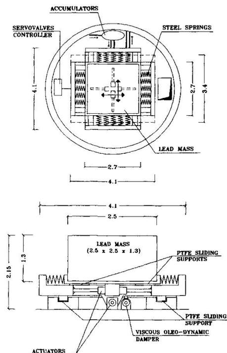
Fig.2 Control device
