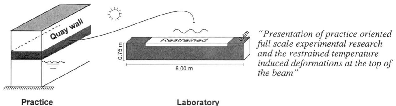
Variables in this study are the level of restraint in specimens, temperature, cement type and curing conditions. All concrete specimens, including large beams and small cubes, are subjected to alternate wetting and drying cycles to simulate the marine condition. In addition, temperature variations are applied to some specimens. In total 90 complete exposure cycles of wetting and drying plus heating and cooling are applied to large beams (from one side) and to small cubes. The
