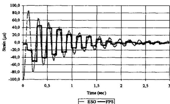
Fig. 5 Time domain signal of the FPS
