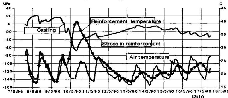
temperature changes of the reinforced concrete structure because of slow warming up and cooling down of concrete. Therefore, for example, on 16 May 1996, the measured air temperature differed from 18 to 27°C degrees ( $\Delta T_{\text{air}}=9^{\circ}\text{C}$ ), and the concrete temperature from 20,5 to 24,5 C ( $\Delta T_{\text{concrete}}=4^{\circ}\text{C}$ ).
