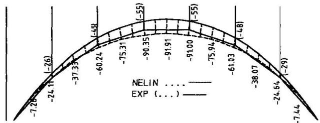
Figure 2 shows differences in displacements between the completed arch and the end of the bridge construction. The displacement difference is determined geodetically and by NELIN program. Comparing experimental and theoretical values of displacements at the all places of the pier and arch junction, averagely 28% higher theoretical values have been obtained.
