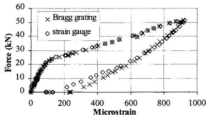
Fig.2 Four point bending test on a concrete prism
