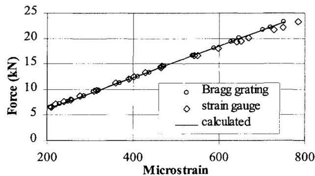
Fig.1 Tensile test on a rebar ( $\phi = 14$  mm)
