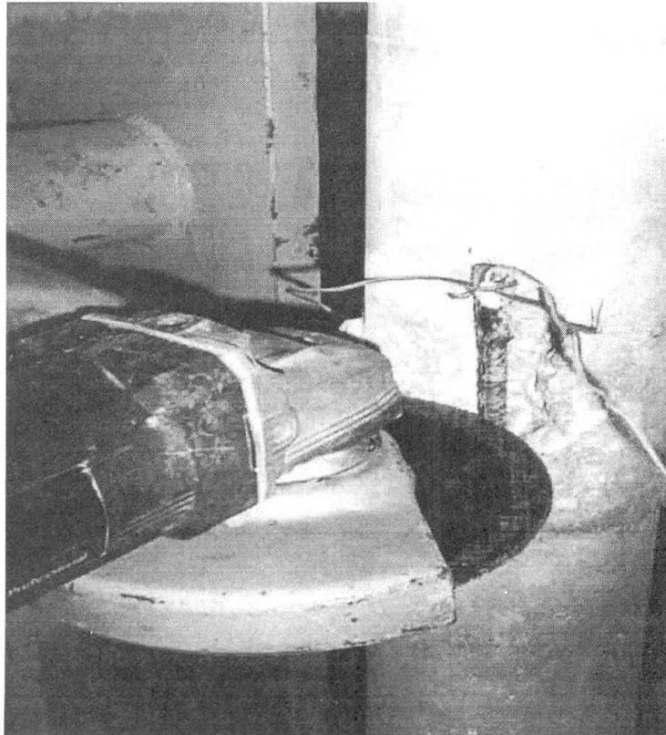
*Fig.1 Electrical saw cutting the bar [1]*
