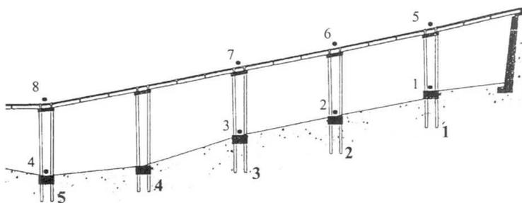
Fig. 2 Sensor locations in configuration A
