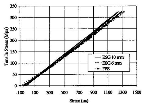
Fig. 1 Stress-strain curves for the steel plate
