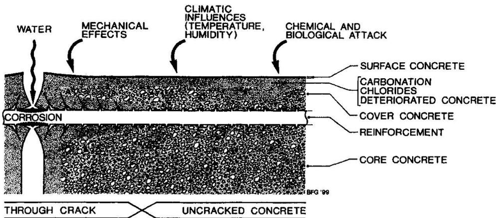
*Fig. 1 Vulnerability of reinforced concrete*
