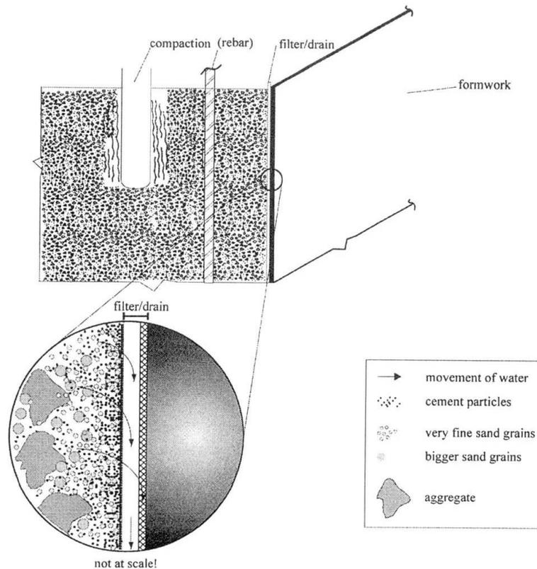
Fig. 1 - Controlled Permeability Formwork - a schematic representation.
