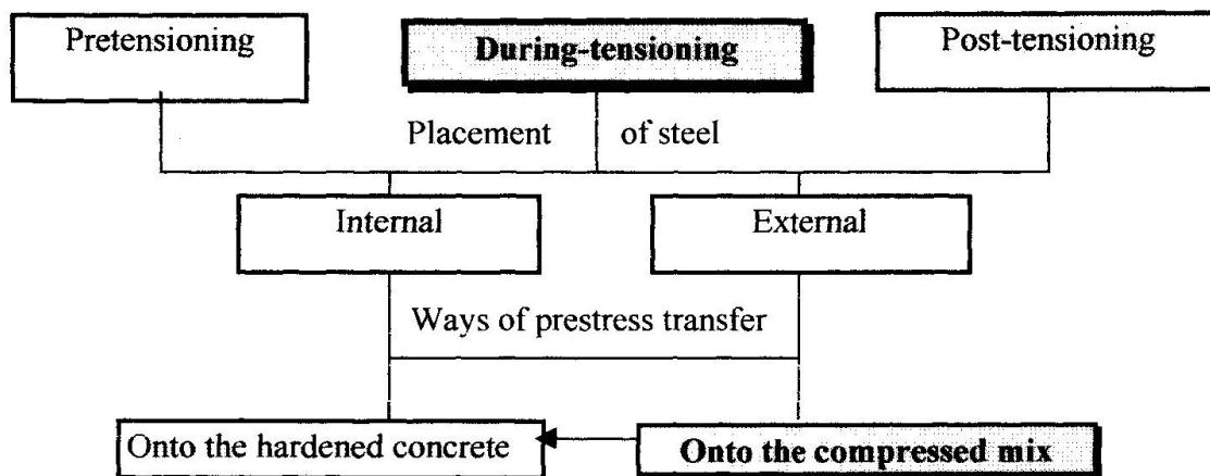
Fig.1. Extended scheme of methods of making prestressing in reinforced concrete structures
