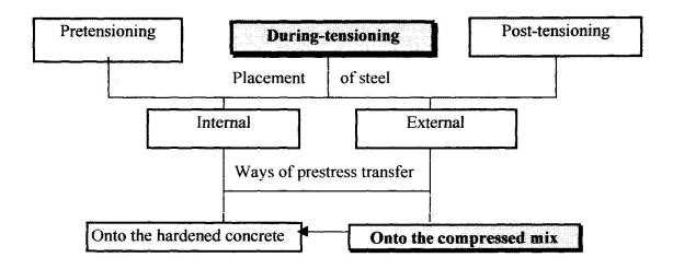
Fig. 1. Extended scheme of methods of making prestressing in reinforced concrete structures
