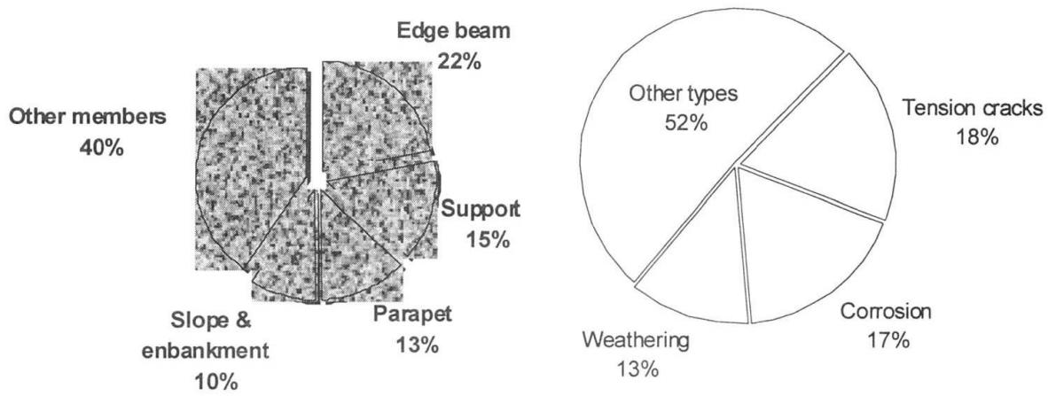
Fig. 5 *Percentage distribution of the damage types remarks on the bridges' different structural members, all condition classes.*
