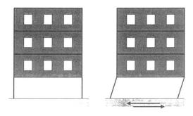
Figure 2: Typical soft storey structure.
