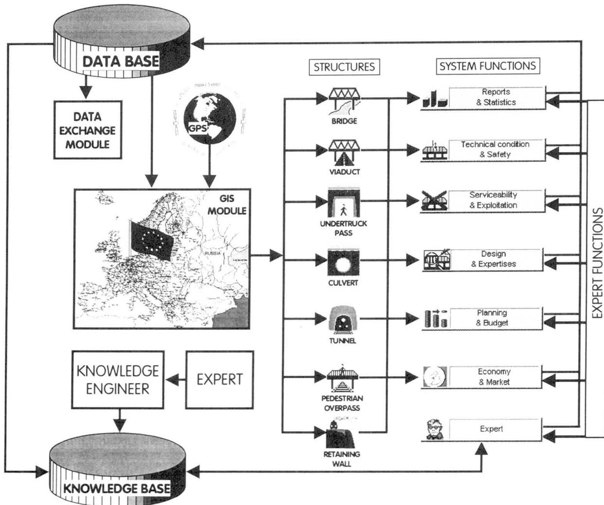
Fig. 1 Functional scheme of the computer part of the ECOBRIDGE System
