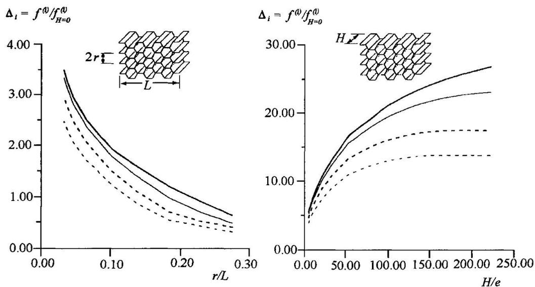
Fig.1 Frequency ratio  $\Delta_i$  versus hexagonal cell ratio  $r/L$  for aluminium honeycomb plate. Frequency mode: (—) 1<sup>st</sup>; (—) 2<sup>nd</sup>; (---) 3<sup>rd</sup>; (-----) 4<sup>th</sup>.
